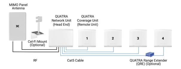
Cel-Fi QUATRA can be installed off-air to provide high-quality in-building wireless connectivity by using the existing cellular network. Off-air installations comprised of an NU and up to four (4) distributed CUs dynamically networked into a single system to provide high-quality in-building wireless connectivity.
