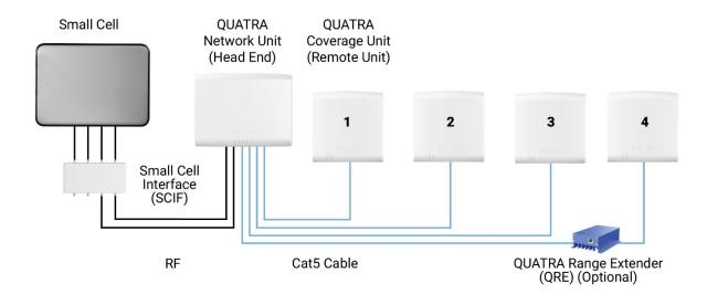
A Supercell is comprised of a Cel-Fi QUATRA 1000 system connected to a small cell. Multiple Cel-Fi QUATRA 1000 systems can be connected to a single small cell, or multiple small cells, to form a coordinated Supercell that extends coverage for large venues. A Supercell with multiple Cel-Fi QUATRA 1000 coverage units (CUs) is more efficient than multiple small cells, and the CUs of a Cel-Fi QUATRA 1000 system connected to a Supercell do not interfere with one another.
