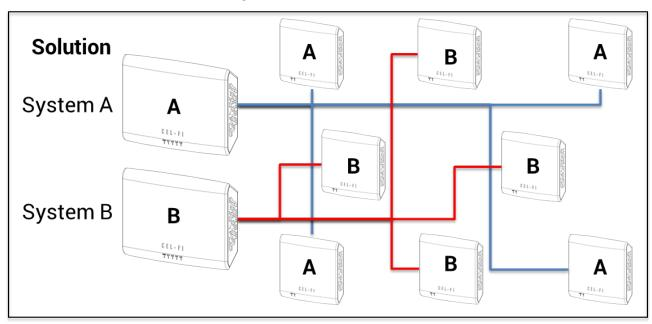
A QUATRA **system** is comprised of a Network Unit (NU) and one to four Coverage Units (CU). An NU and CU are paired; they must be of the same model, and band configuration. Multiple QUATRA systems can be installed together to form a larger **solution**. Systems can be attached to a specific **site** in WAVE, and managed accordingly. A site represents a physical location, in WAVE; an address.
